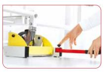
The patented lift mechanism permits placement of the load cells without any effort.
